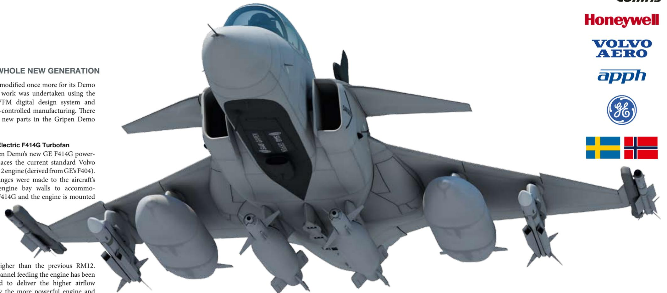
by SAAB and Thales Norway, will take Gripen's netcentric capability to a new level. Gripen Demo is also fitted with a broadband UHF video datalink, for use with ground forces, allowing the aircraft to communicate most effectively with forward air controllers in the Close Air Support role.
